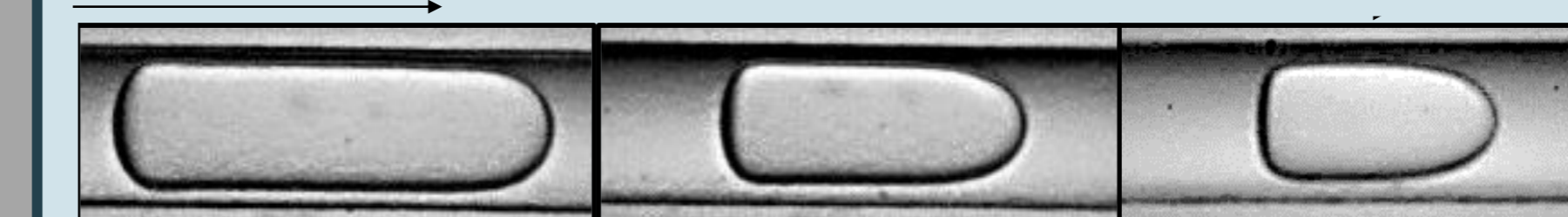
Images of plugs with increasing mixture velocity in 0.5 mm channel
